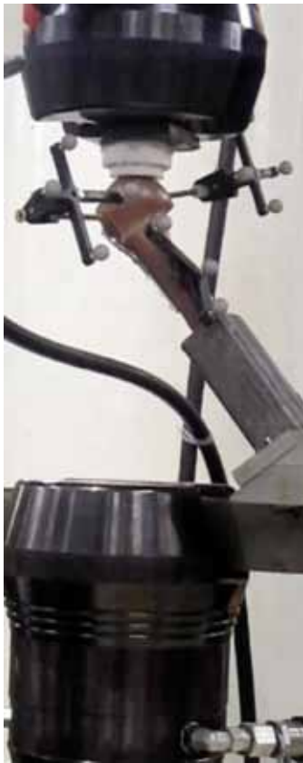
Figure 3 The bio-mechanical testing model with the Optotrak sensors.
