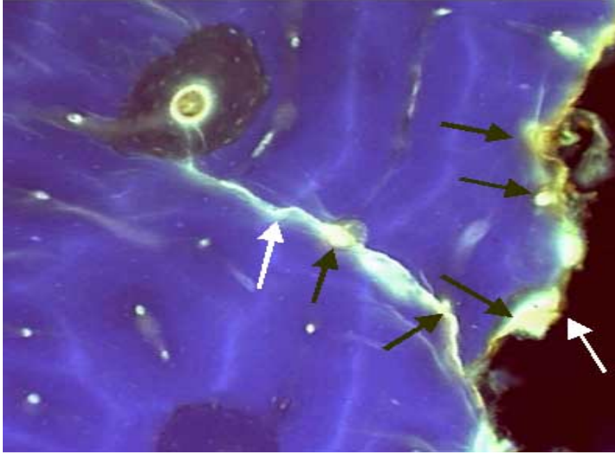
Fig. 5. This illustrates a typical example of two large cracks (white arrows) that were involved in failure of a specimen (the second crack is the main failure surface). As these cracks grew to macrocrack size, they managed to penetrate the cement lines of numerous osteons and used the Haversian canals (black arrows) as weaknesses in which to further propagate.
